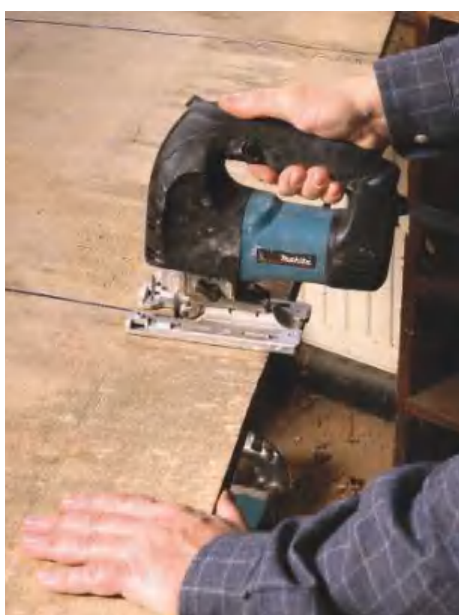
▲ Pic.16 Portable power tools such as this jigsaw are good for roughing out wood before finally trimming to size with a hand plane or machine
